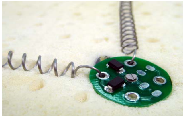
figure 3. Detail of circuit board and SMA coils
