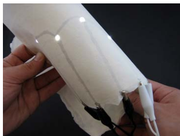
figure 2. Composite combining natural paper and electronic components [2].
